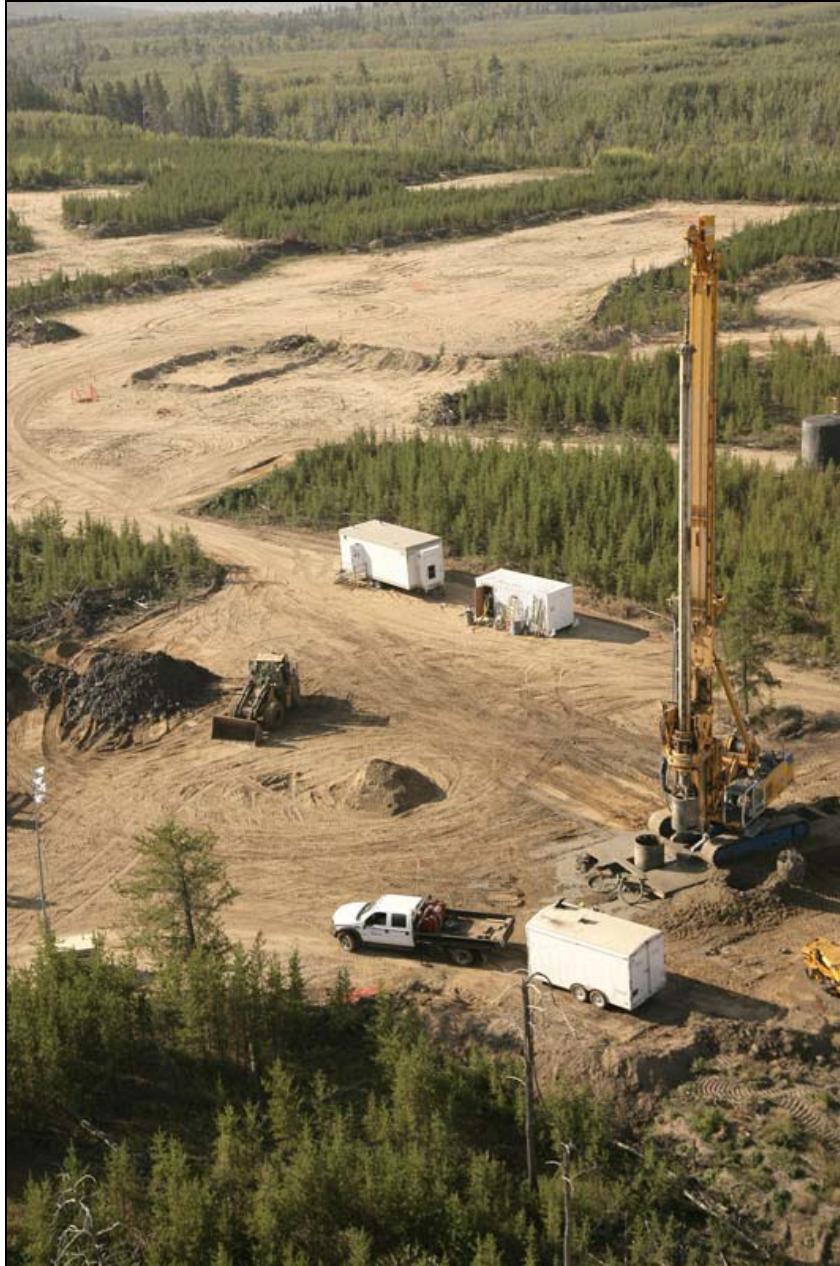
Figure 11-2: LDD Rig in Kelly Drill Mode
