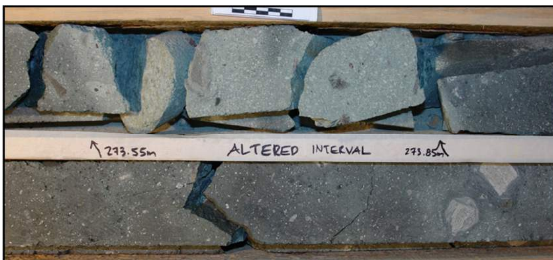
Figure 7-8: Example of Typical Matrix-Rich Pense Kimberlite with a More Altered (Lighter) Domain and a Less Altered (Darker) Domain (From 141-06-071C: 273.55 m) (from Harvey, 2011)
