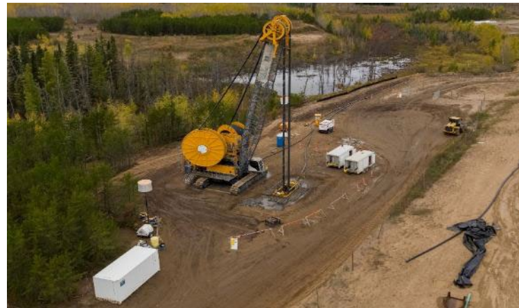
RTEC trench cutter bulk sampling rig
