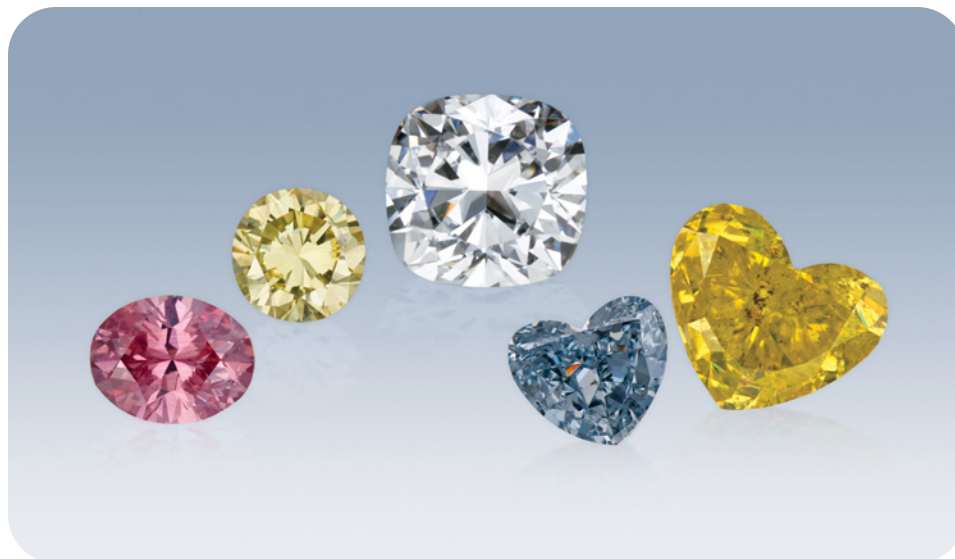
Figure 1. Gem diamonds such as these are prime examples of their respective diamond types (from left): 0.47 ct type Ia pink, 0.38 ct type Ia “cape” yellow, 1.04 ct type IIa colorless, 0.56 ct type IIb blue, and 1.01 ct type Ib “canary” yellow. All the colored diamonds are part of the Aurora Butterfly of Peace collection. Composite photo by Robert Weldon and Kevin Schumacher.
